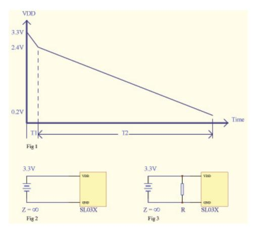
SL030/SL031/SL032 will can't run correctly when power-cycling appearing during T2. In extreme conditions, there are no any discharge components in the circle as Fig 1. T1 = 20us, T2 = 2.2s
