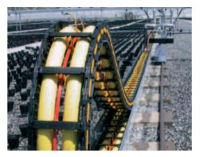
Specialist for operation on very long travelling distances up to 400 meters. Chain links with shoes made of lowfriction, low-wear plastics. System-completing channel constructions available for supporting and guiding the chain.
