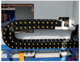
All purpose, due to its single pin, also for higher mechanical requirements. Specially for small and medium-size chains. Available closed or with foldable lid.
